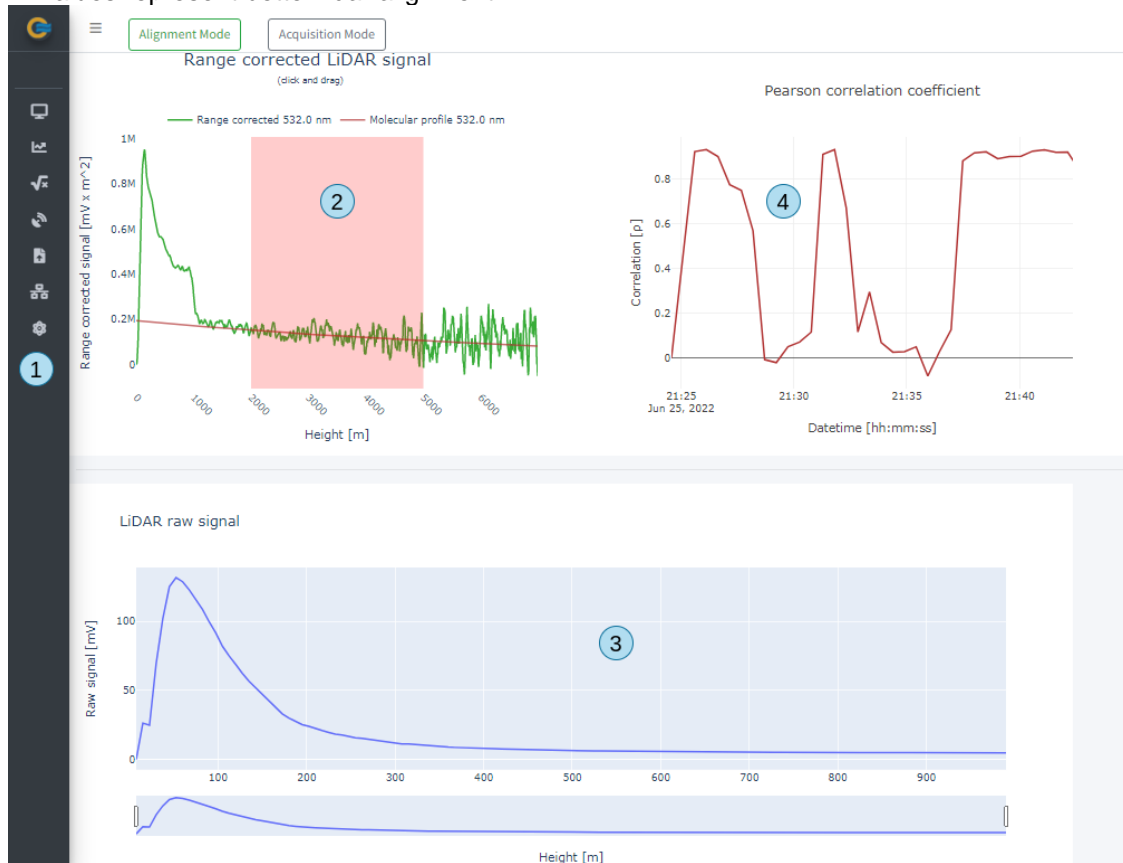
Figure 1 - General view of the dashboard. (1) Settings panel. (2) Range corrected lidar signal (RCLS, green line) and its Rayleigh-Fit (red line). (3) raw lidar signal. (4) alignment-quantification plot, where higher values represent better lidar alignment
