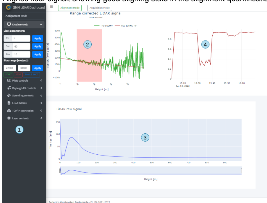
In panel 4 of Figure 3 can see the historic time series of the cross-correlation coefficient. Since lidar signals are inherently noisy, and despite the fact that this coefficient is
